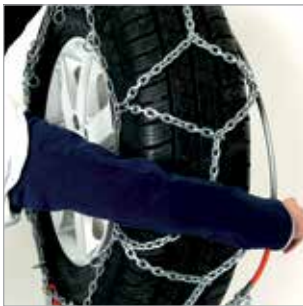
RUDmatic® hoop fitting Easy fitting thanks to a strong springsteel hoop. Especially easy to fit on rearwheel drives.
